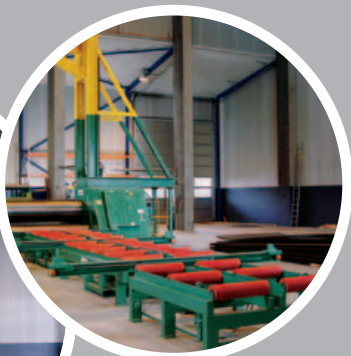
PAS 700 with top support, side support and infeding table
