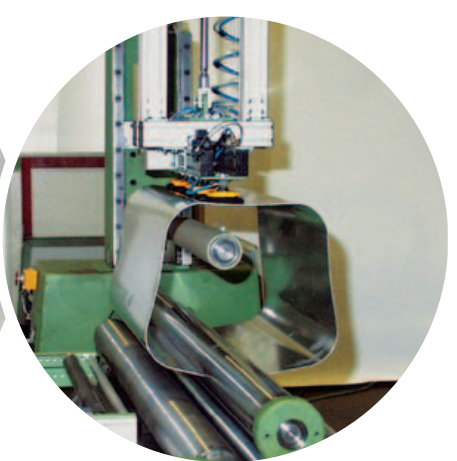
Automatic outfeeding of finished tank body
