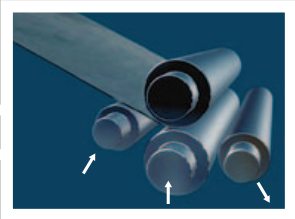
2. Raise the front side roll. Prebend and roll.
