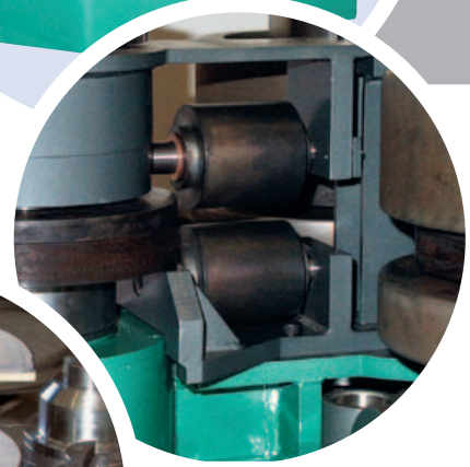
R-6 with special guide unit for bending I & U-beams, hard way
