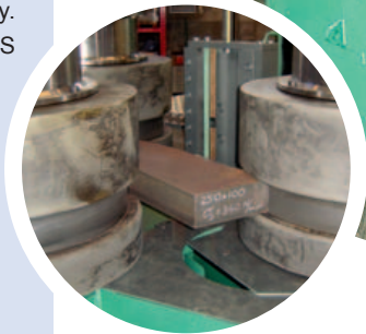
R-14-S Bending flat bar 250x100 mm (10" x 4")
