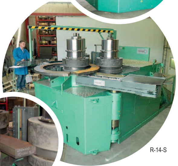
R-14-S Bending flat bar 250x100 mm (10" x 4")
