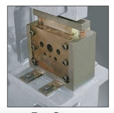
ROD SHEAR For a more precise cut on your round stock sizes 1/4", 3/8", 1/2", 5/8", 3/4", 1"
