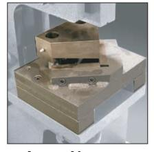
ANGLE NOTCHER Tooling takes a precise 92° notch from the bottom leg of angle iron up to 3" x 3" x 1/4" maximum
