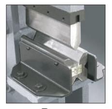
BRAKE In 7", 8", 10" and 12" lengths\* — includes a standard "punch" and a four-way die for braking 1/16", 1/8", 3/16", and 1/4" material to a 90° angle
