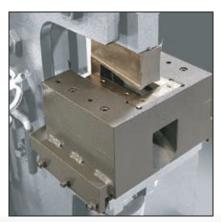
**COPER/NOTCHER** Allows for a small "nibble" or a large notch to be taken out of plate, bar stock, or angle\*
