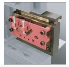
MULTI SHEAR Angle Shear: 2" x 2" x 1/4" Bar Shear: 1/4" x 6" Rod Shear / Round: 1/4", 3/8", 1/2", 5/8", 3/4" Rod Shear / Square: 13/16"
