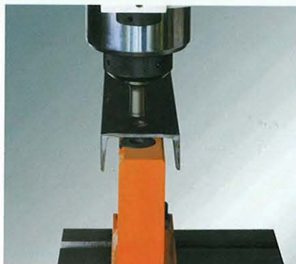
Single hole die holder for punching channel webs. (optional on double cylinder models)
