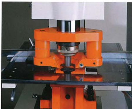
*Urethane spring stripper for minimal deformation.
