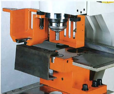
Standard overhung die holder for punching channel flanges and angles. (optional on single cylinder models)
