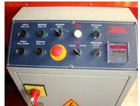
Control Panel featuring a Digital Readout
