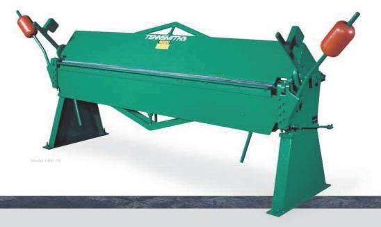
TENNSMITH's heavy-duty hand brakes are designed and built for long service and accurate bending. Welded steel plate construction and heavy truss rods and braces provide strength and durability.
