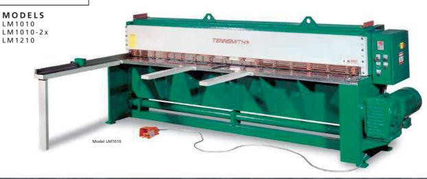
TENNSMITH's LM1010 is equipped with a standard "GO TO" 30-inch back gauge system. The ballscrew-driven back gauge provides quick, accurate cuts. The LM1010 is powered by a 12-1/2-hp gear motor attached to a mechanical linkage which provides smooth, quiet operation.
